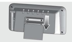
Batteries serve as back-up only. Use 3 pieces of AA (UM-3) 1.5V batteries. Insert batteries, matching the polarity. Press **RESET** after each battery change.
